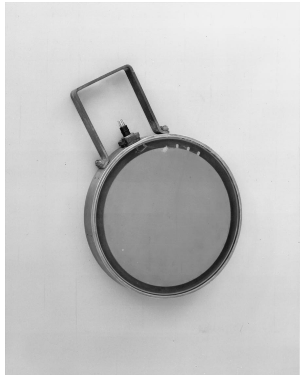
FIG. 3. Injection-molded 1–3 piezoelectric composite transducer standard (F82).
